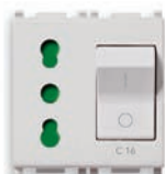
14273 (.SL) Bpresa SICURY 2P+T 16 A P17/11 250 V~, 1P+N C 16 - 2 moduli
