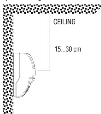
Methane gas is lighter than the air and therefore rises and it concentrates in the highest point of the room.
