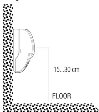
As LPG is heavier than air and it is deposited in layers in the lower part of the room, the greatest concentrations are first found near the floor. The detector must be placed at 30cm approx. from the lowest stepping level. The detector must not be placed near exits or on the floor. Do not install the detector on the floor. Do not place the detector in areas where it can be damaged by involuntary shocks (as during normal household cleaning, washing etc.).
