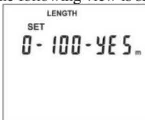
4. Press SET/UNIT to select the 0-9 marker and again SET/UNIT to set the length  $10 \div 250$  (unit m) or  $30 \div 750$  (ft unit). The value flashes to display. Use the indicator keys
