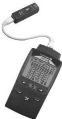
5. Press the key
