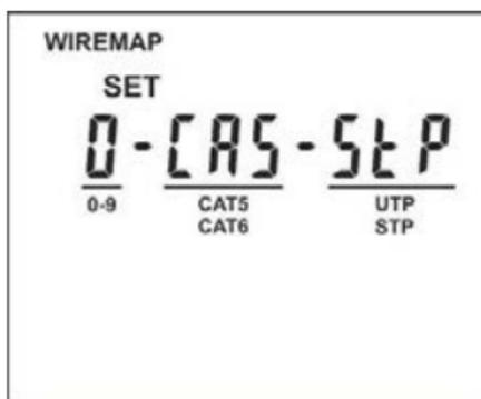
4. Press the SET/UNIT button. Parameter "0" flashes to display. this parameter allows you to select one of the numeric configurations from 0 to 9 saved by the user based on the type and whether the cable length is calibrated
