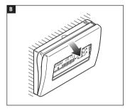
The letters  $b\vec{a}b\vec{b}$  on the display means that the batteries are flat and must be replaced.
