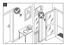
Install the unit in a position which is suitable for correct room temperature measurement, for example on an internal wall. Avoid installation in alcoves, behind doors or curtains, or near heat sources.
