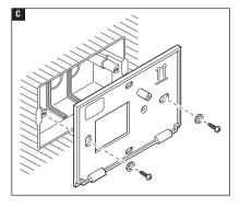
Fasten the base to the wall or to the recessed back-box, passing the connection cables through the opening for this purpose and respecting the sign showing which way is UP .
